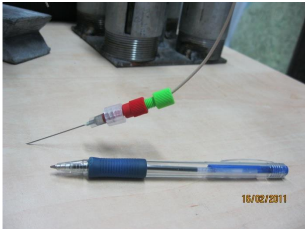
Fig. 2. VacuSIP with male Luer connector intended for large collecting containers such as penicillin or EPA bottles.
