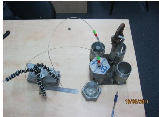
Fig 3. The entire setup with 100 mL penicillin bottles in a costume made carrier. The Peek tubing is attached to a weighted Joby Gorillapod GP1 ( http://joby.com/gorillapod/original ) that allow excellent manoeuvrability and exact positioning of the tube inlet
