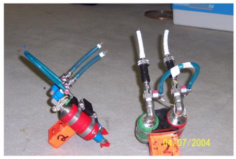
The SIP is a new water sampler designed to allow clean point source water sampling. A simple valve operation by an ROV manipulator or a SCUBA diver allows the external water pressure to force the sampled water into a Teflon coated stainless steel sample cylinder. The small ID of the inlet tube (capillary PEEK) insures slow suction rate during the sampling.
